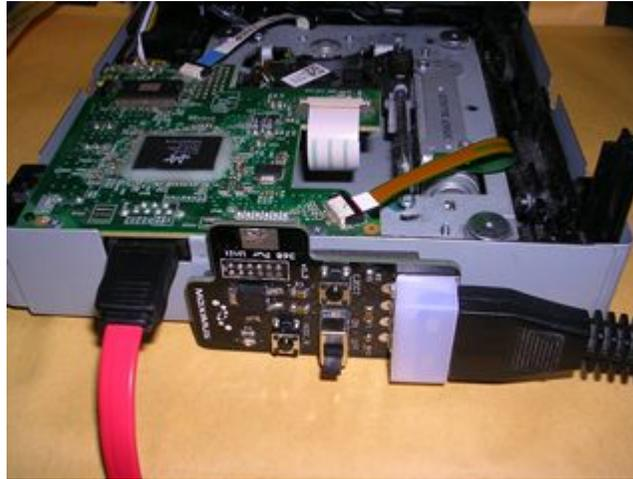
*Sata and Power cables connected, use croc clip cable if needed*
