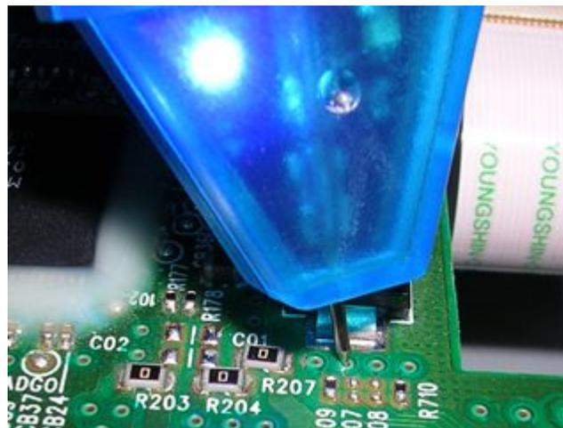
*TX spot contacted by the probe, blue led will light up as visual confirmation*
