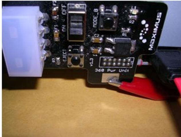
*The croc clip cable connected on the ground spot, the other end of the croc clip goes to your PC chassis*
