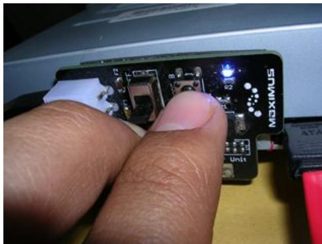
*To start Modeb on hitachis, press Modeb button while turn on switch, release modeb after 2 seconds*
